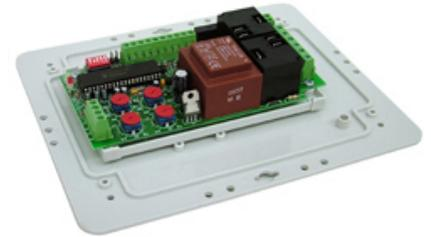
The **EC-300** Energy Controller eliminates energy waste in any room while no replacement or adjustment of the existing HVAC or lighting systems is required.
